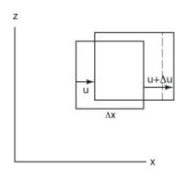
Normal strains are defined as change in length divided by the original length. So here, normal strain in the x-direction, written  $\varepsilon_{xx}$ , is:
