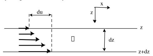
If the velocity does not change along the along the length of the channel (ie  $\partial u/\partial x = 0$ ) then stress along a horizontal plane is related to the velocity gradient by:
