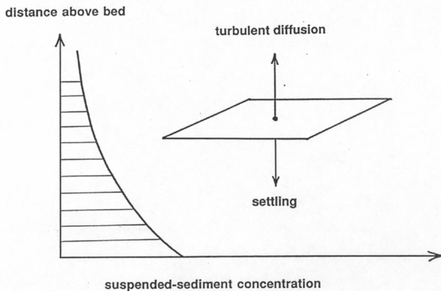
**Figure 2-33** Vertical balance between downward settling and upward turbulent diffusion in suspended-load transport
