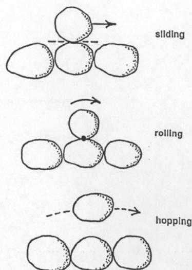
**Figure 2-31** Modes of bed-load movement
