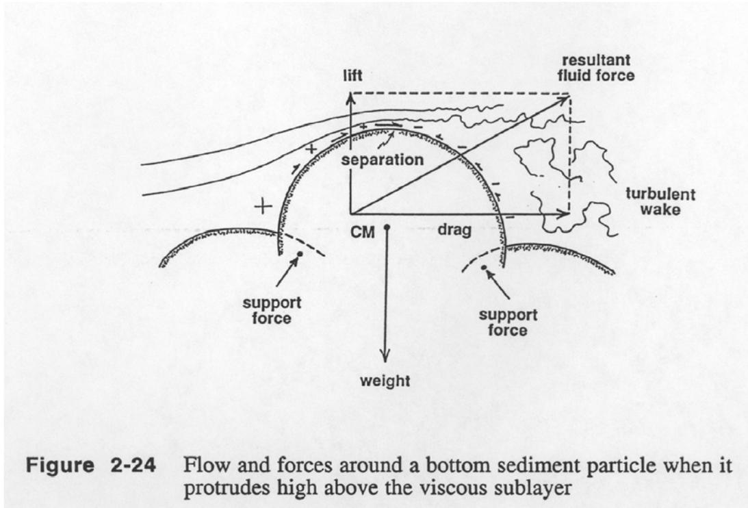
**2.2.8** Note in Figures 2-23 and 2-24 that because the pressure is relatively low at the top of the hemisphere and relatively high around its base, there's a **lift** component to the resultant force. This is exactly the same kind of lift force that acts on airplane wings. The lift force can be almost equal to the downstream component of the resultant force (which is called the **drag**).
