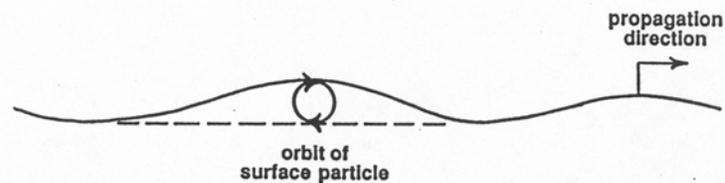
**Figure 2-16** The circular orbit of a surface particle floating on the water surface as a wave passes
