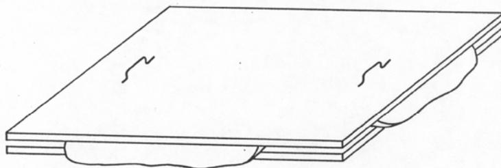
Figure 2-1 Shearing a viscous fluid between two parallel plates
