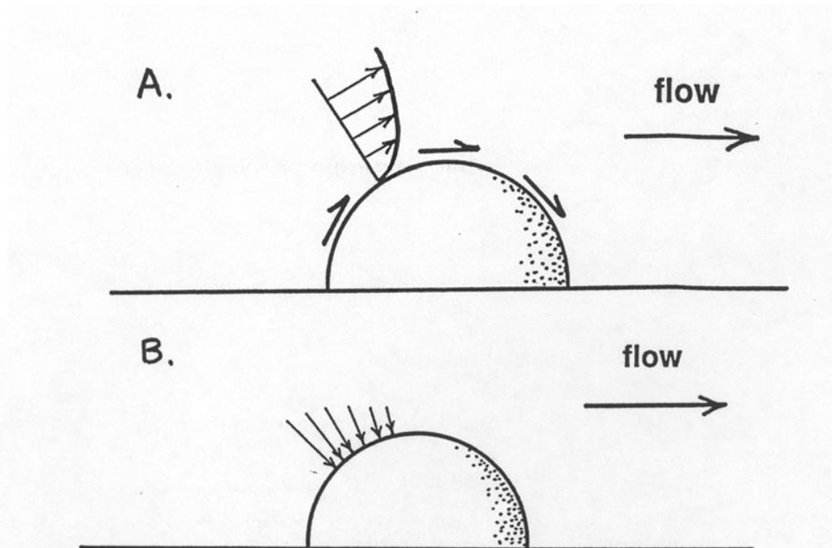
**Figure 2-21** A: viscous forces acting on the surface of a hemisphere on a planar boundary exposed to a flow. B: pressure forces acting on the surface of a hemisphere on a planar boundary exposed to a flow
