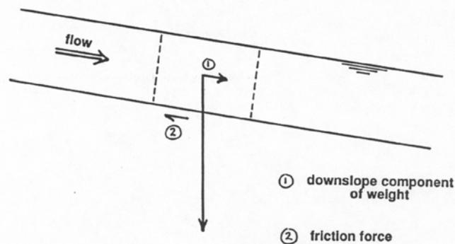
**Figure 2-5** In a flow down a sloping channel, the weight of an element of fluid has a downslope component that's balanced by the friction force the boundary exerts on the flow
