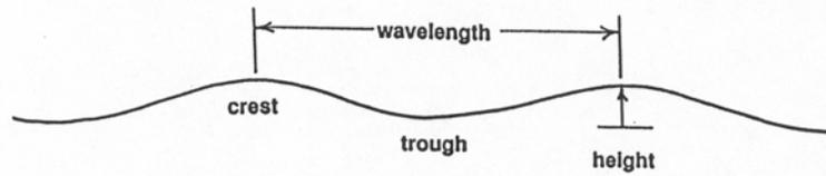
**Figure 2-15** Some terms used to describe the waves in a simple train of waves
