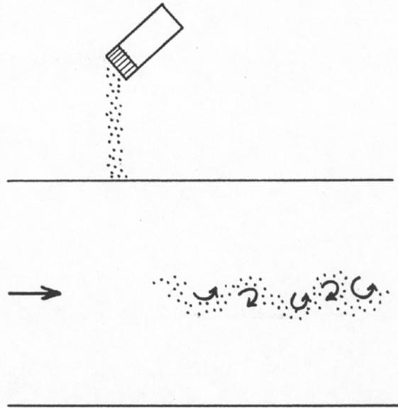
**Figure 2-11** Sprinkling the flow with magic powder that allows you to see the eddies
