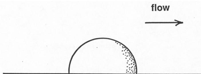
**Figure 2-20** Flow around an isolated hemisphere on an otherwise planar boundary
