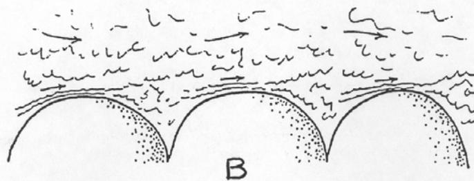
Figure 2-13 A: dynamically smooth flow B: dynamically rough flow
