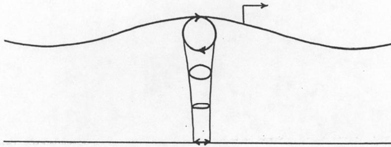
**Figure 2-18** Decrease in orbit diameter with depth beneath a shallow-water wave
