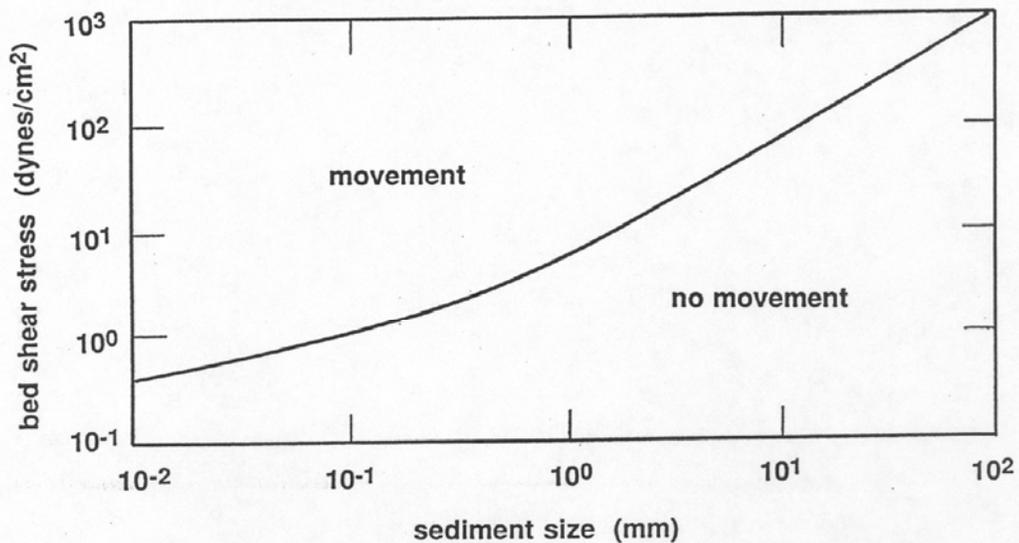
**Figure 2-25** Threshold curve for incipient movement of quartz sediment in water
