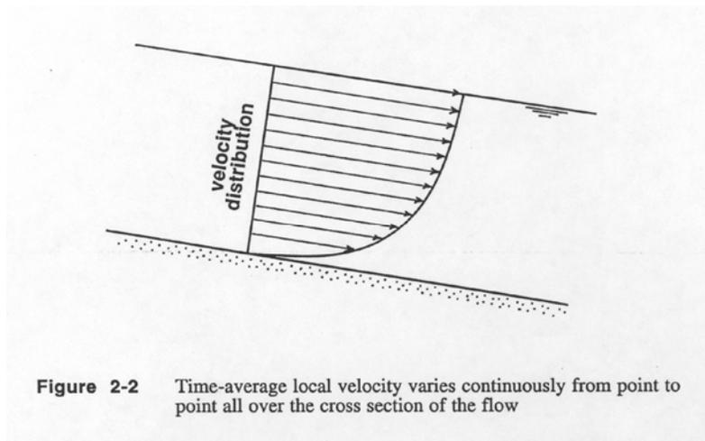
**1.2.6** You can take the average of all the local velocities all over the flow cross section to get a *mean flow velocity*  $U$  (Figure 2-3). In real rivers this is how it's actually done, but in laboratory channels, where it's easy to know the water discharge (the volume rate of flow), you can use the relationship  $Q = UA$ , where  $Q$  is the discharge and  $A$  is the area of the flow cross section, to find  $U$ .
