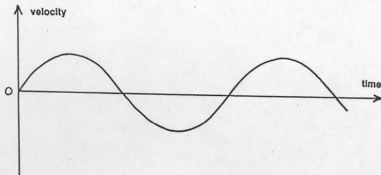
**Figure 2-19** Fluid velocity near the bottom as a function of time at a point that's fixed relative to the bottom, as a shallow-water wave passes by overhead
