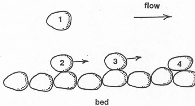
**Figure 2-30** Particles that belong to the bed and that belong to the load. Particle 1 is part of the flow. Particle 2 has just come into contact with the bed but it's still moving so it's part of the flow. Particle 3 has just been set into motion, so it's part of the flow. Particle 4 is exposed to the flow but is at rest so it's part of the bed.
