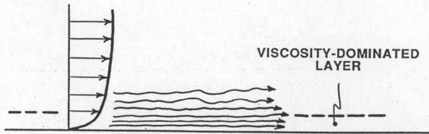
**Figure 2-12** The viscosity-dominated layer at the base of a turbulent channel flow
