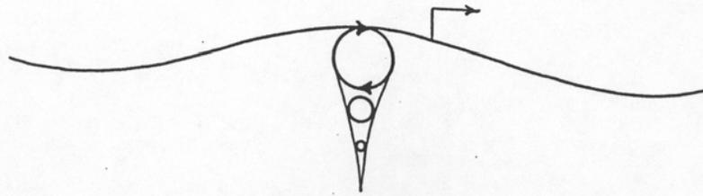
**Figure 2-17** Decrease in orbit diameter with depth beneath a deep-water wave
