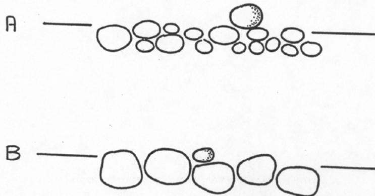
**Figure 2-38** Exposure/shielding effect in mixed-size sediment transport. A: Larger particles tend to be exposed to the force of the flow. B: Smaller particles tend to be shielded from the force of the flow.
