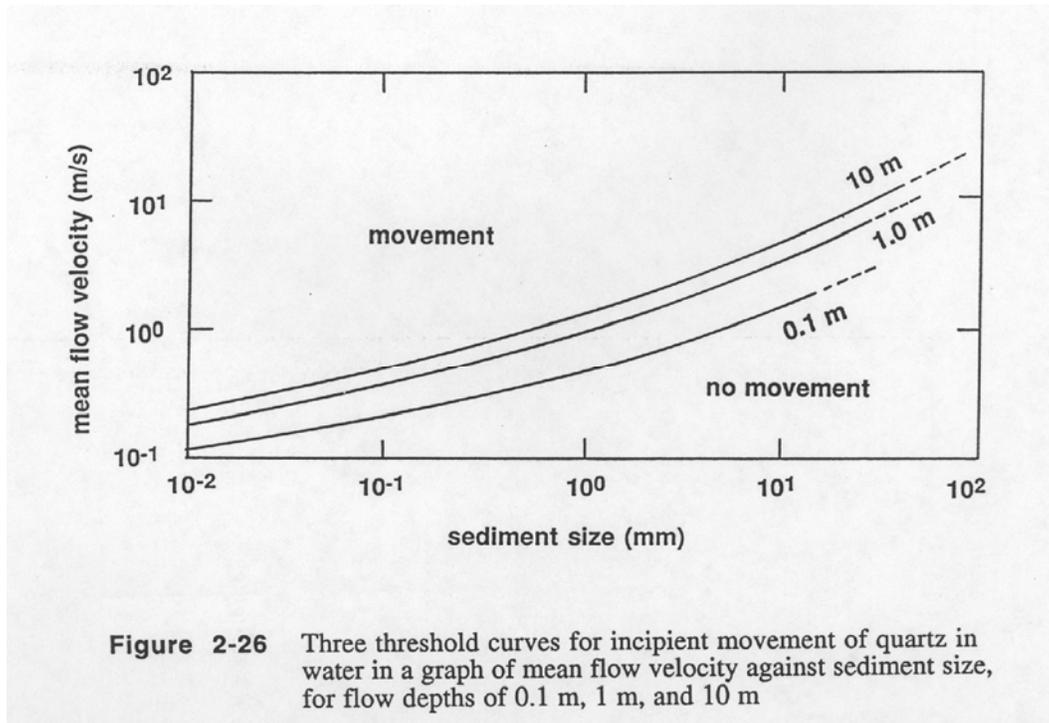
**Figure 2-26** Three threshold curves for incipient movement of quartz in water in a graph of mean flow velocity against sediment size, for flow depths of 0.1 m, 1 m, and 10 m
