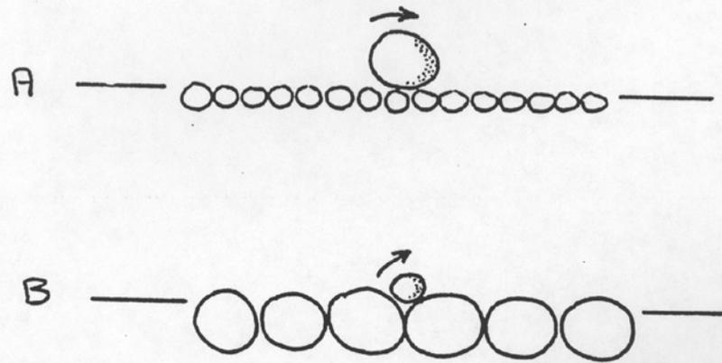
**Figure 2-39** Rollability effect in mixed-size sediment transport. A: Larger particles roll easily on a bed of small particles. B: Smaller particles roll with difficulty on a bed of larger particles.
