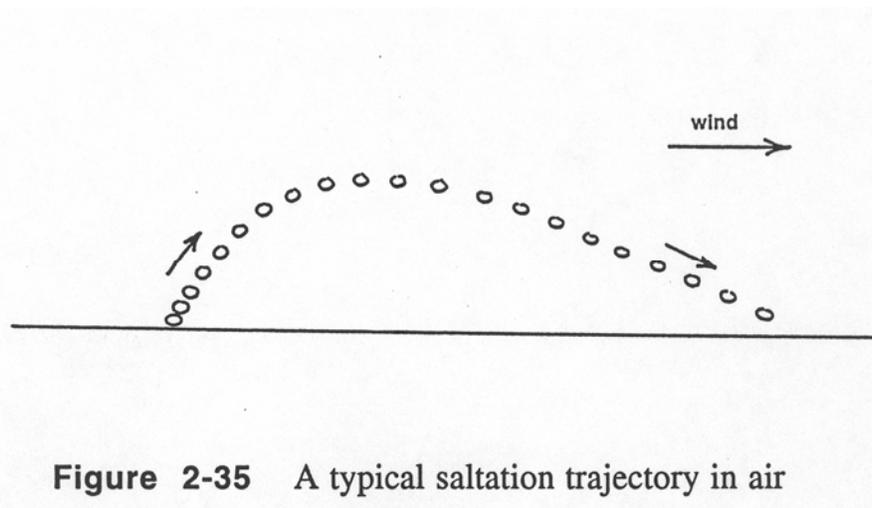
**Figure 2-35** A typical saltation trajectory in air
