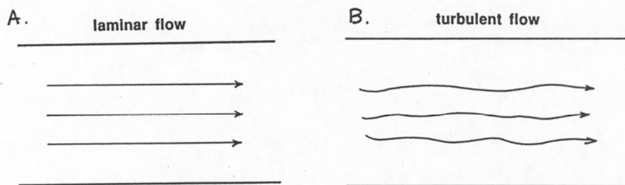
**Figure 2-8** Paths of fluid elements in laminar and turbulent flow
