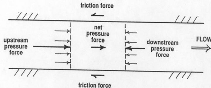
**Figure 2-6** In a flow in a horizontal pipe or conduit, the fluid moves only if there's a downstream decrease in fluid pressure
