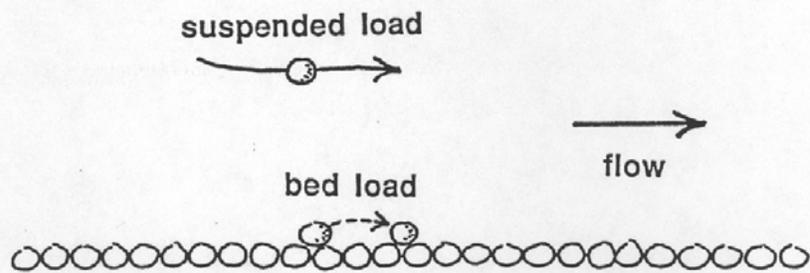
**Figure 2-28** Bed load and suspended load
