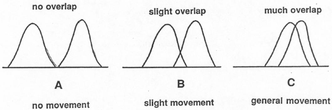
**Figure 2-27** Threshold condition viewed in terms of two probability distributions. In each sketch, the curve on the left shows the distribution of instantaneous local fluid forces on bottom sediment particles, and the curve on the right shows the distribution of instantaneous fluid forces needed to set the bed particles in motion.
