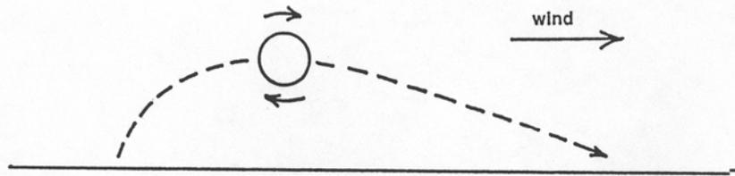
**Figure 2-37** Spin of a particle saltating in air
