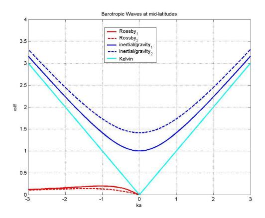
In the above, we have scaled the horizontal wavenumbers by the radius of deformation, and the frequency by the inertial frequency. We have chosen a couple of wave modes of each type by setting the scaled meridional wavenumber (la) to be 0 or 1.
