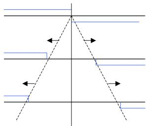
Eventually, there will be a flat interface in the field of view but the fluid will still be moving from left to right as the "far field" adjusts to the initial disturbance. This is an example of waves in a non-rotating system.
