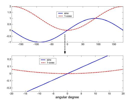
We now insert into the above the fact that  $\theta = \theta_0 + \theta'$ , where  $\theta' << 1$ , & use the trigonometric identity for sin(a+b)=sin(a)cos(b)+cos(a)sin(b). Now as seen in the above figure, for small angular changes (expressed in radians) from the reference latitude,  $cos(\theta') \sim 1$  &  $sin(\theta') \sim \theta'$ .
