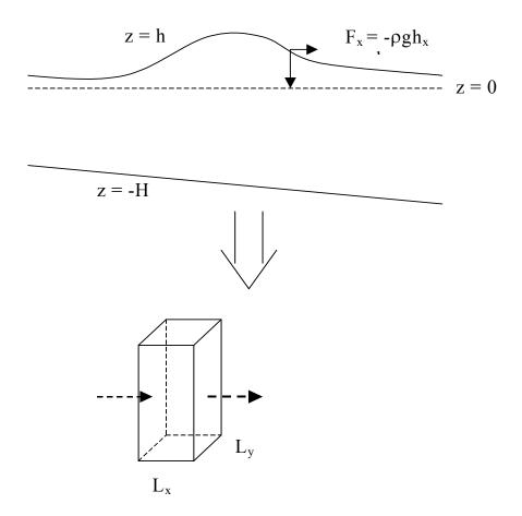
$uL_{y}(H+h)_{rhs} - uL_{y}(H+h)_{lhs} = L_{y}\Delta[u(H+h)] = \text{net loss of fluid in x-dir.}$  $vL_{x}(H+h)_{front} - vL_{x}(H+h)_{back} = L_{x}\Delta[v(H+h)] = \text{net loss of fluid in y-dir.},$
