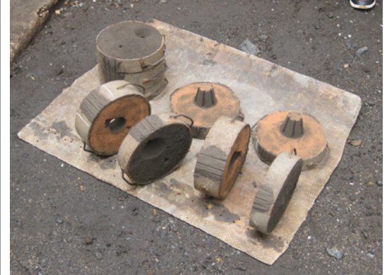
Molds for sandcasting a corn sheller at Suame Magazine, Ghana, Africa.
