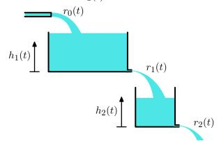
The rate of flow out of each tank is proportional to the height of the water in that tank:  $r_1(t) = k_1 h_1(t)$  and  $r_2(t) = k_2 h_2(t)$ , where  $k_1$  and  $k_2$  are each  $0.2 \,\mathrm{m}^2/\mathrm{second}$ . Both tanks have heights of 1 m. The cross-sectional area of tank 1 is  $A_1 = 4 \,\mathrm{m}^2$  and that of the second tank is  $A_2 = 2 \,\mathrm{m}^2$ . At time t = 0, both tanks are empty.
