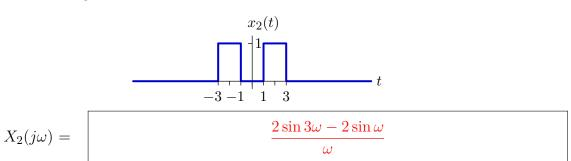
$$X_2(j\omega) = \int_{-3}^{-1} e^{-j\omega t} dt + \int_{1}^{3} e^{-j\omega t} dt = \frac{e^{-j\omega t}}{-j\omega} \Big|_{-3}^{-1} + \frac{e^{-j\omega t}}{-j\omega} \Big|_{1}^{3}$$
