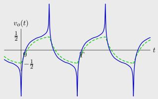
The asymmetry in the "charging" and "discharging" portions of the RC response is even more pronounced than before. Because the magnitudes of the higher harmonics are not attenuated, they now accumulate to make a substantial peak that was not seen in the RC response. We can understand the large overshoot as follows. Each harmonic component in the square wave is a sinusoid:
