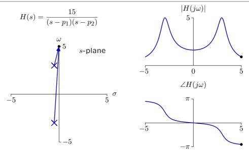
Consider the system represented by the following poles. s-plane  $\omega_d$  $\sigma$  $\omega_d$ Find the frequency  $\omega$  at which the magnitude of the response y(t) is greatest if  $x(t) = \cos \omega t$ . 1.  $\omega = \omega_d$ 2.  $\omega_d < \omega < \omega_0$
