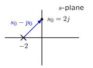
The denominator of  $H(s)|_{s=2j}$  is 2j+2, a vector with length  $2\sqrt{2}$  and angle  $\pi/4$ . Therefore, the response of the system is
