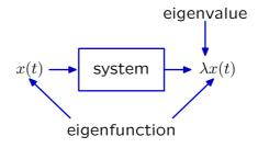
Consider the system described by  $\dot{y}(t) + 2y(t) = x(t)$ . Determine if each of the following functions is an eigenfunction of this system. If it is, find its eigenvalue.
