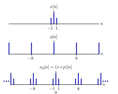
Convolution by an impulse train in time is equivalent to multiplication by an impulse train in frequency.
