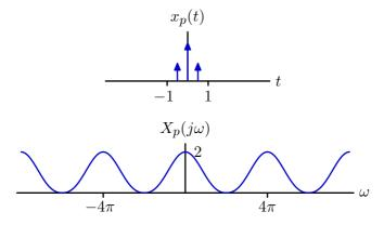
Fourier transform of sampled signal  $x_p(t)$  has same shape as DT Fourier transform of x[n].
