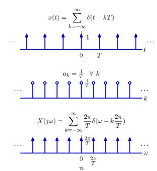
Easier to calculate z(t) by convolving x(t) with an impulse train.
