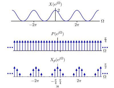
Periodic extension of a discrete signal (x[n]) results in a signal  $(x_p[n])$  that is both periodic and discrete. Its transform  $(X_p(e^{j\Omega}))$  is also periodic and discrete.
