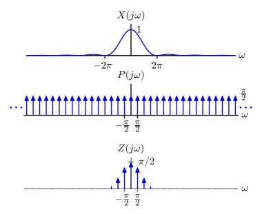
The Fourier transform of a periodically extended function is a discrete function of frequency  $\omega$ .
