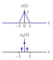
Multiplying x(t) by an impulse train in time is equivalent to convolving  $X(j\omega)$  by an impulse train in frequency (then  $\div 2\pi$ ).
