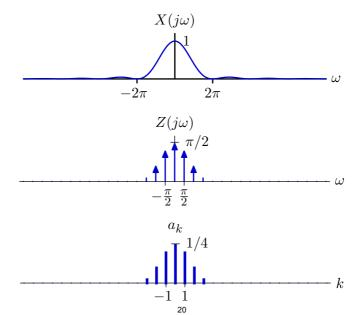
Periodic extension of CT signal  $\rightarrow$  discrete function of frequency.
