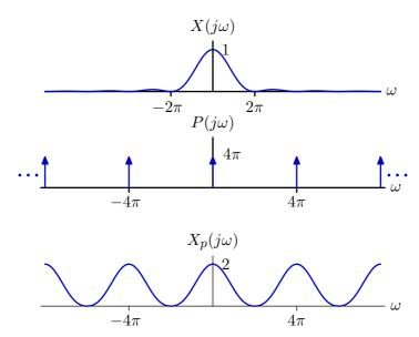
Fourier transform of sampled signal  $x_p(t)$  is periodic in  $\omega$ , period  $4\pi$ .
