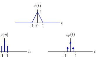
We can generate a signal with the same shape by multiplying x(t) by an impulse train with  $T=\frac{1}{2}.$
