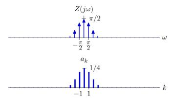
The effect of periodic extension of x(t) to z(t) is to sample the frequency representation.
