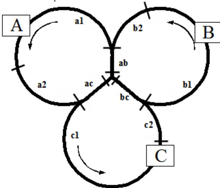
With this setup, each of Alice, Bobby, and Chip have their own trains, and each train travels in a circular path in the indicated (counterclockwise) direction. Note that there is a section of track shared between each pair of trains. In order to avoid sibling battles due to train wrecks, Gill has devised a system for segmenting the track, and has programmed each train to use a semaphore to avoid simultaneous use of the shared track sections **ac**, **ab**, and **bc**.
