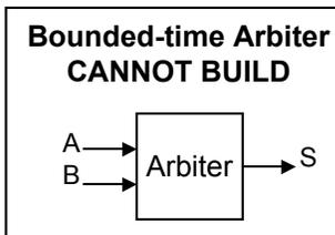
Sample *S* at a specified time after *A* and *B* have risen to find out which rising edge came first – *A* or *B*. The Arbiter may enter a metastable state if *A* and *B* rise at exactly the same time. The Arbiter will eventually come to decision in *unbounded* time but might be metastable and invalid when *S* is sampled.
