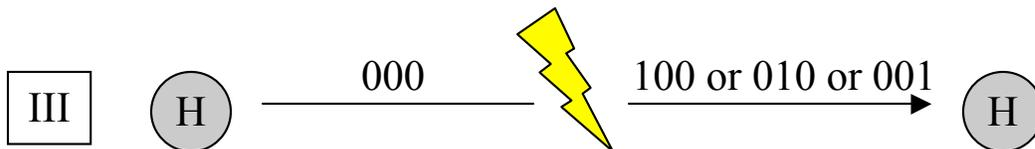
For two encodings of the *same* length, the Hamming Distance (**D**) is the number of bits you need to change to turn one into the other. We increased the Hamming Distance by one in each step of this example. (I)  $D = 1$       (II)  $D = 2$       (III)  $D = 3$ .
