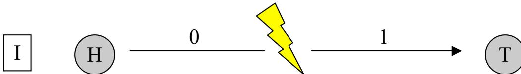
If we increase the number of bits in the encoding to two bits (heads = 00 and tails = 11), we can detect single-bit errors. However, we still cannot correct them.
