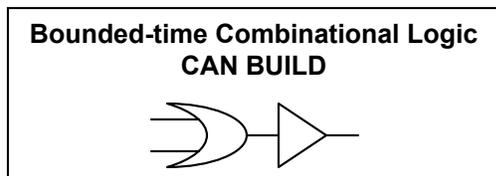
We are guaranteed a valid output after a specified propagation delay.
