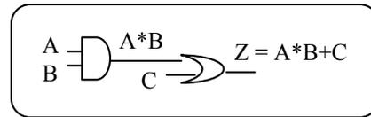
If you wish to derive a logic equation from an existing circuit, try to derive intermediate equations, starting at the inputs and working incrementally towards the output. You can use boolean algebra to manipulate the formula to whatever format you prefer.
