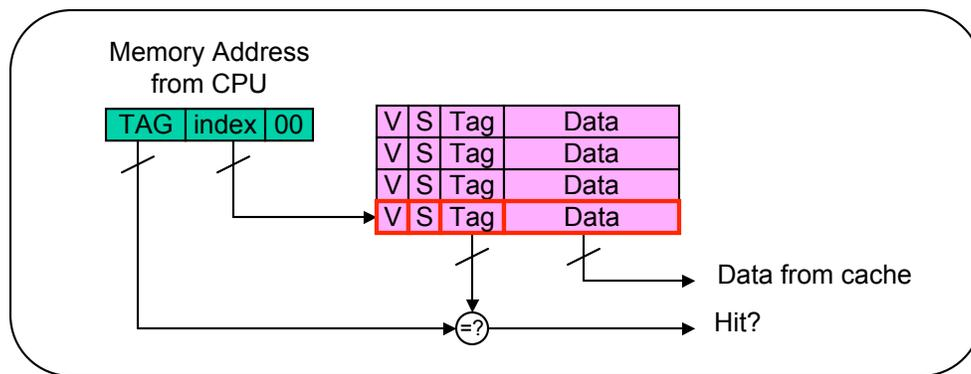
The direct-mapped cache is cheaper than the fully-associative cache because it only has one tag comparator for the entire cache, as opposed to one tag comparator for every line in a fully-associative cache. However, address collisions are possible in a direct-mapped cache, which might adversely affect performance.
