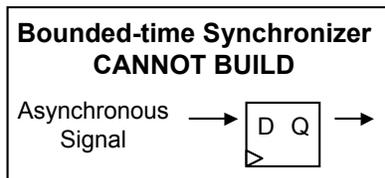
If the *D* input does not meet the flip flop's setup and hold time, the *Q* output might be metastable.
