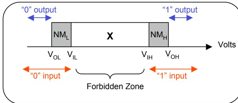
In the digital world, a voltage can represent a valid “0”, a valid “1”, or an invalid signal “X” (a voltage in the forbidden zone). Voltage is continuous, therefore we define boundaries to indicate whether it’s a 0, 1, or X.
