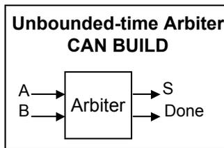
Sample *S* when the *Done* signal is high to find out which rising edge came first – *A* or *B*. *S* may enter a metastable state if *A* and *B* rise at exactly the same time. However, we are guaranteed that *S* will be valid when *Done* is high, therefore *this* arbiter will not cause other metastable states.
