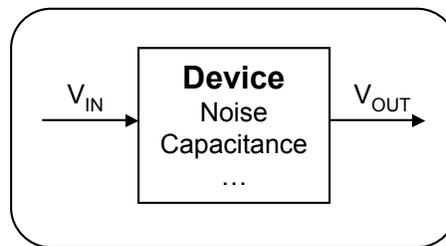
The world is not ideal, however, so we must ensure that a “0” will never be mistaken for anything else. This is done by applying stricter boundaries to the outputs of combinational logic blocks ( $V_{OL}$  and  $V_{OH}$ ) and more lenient boundaries on the inputs ( $V_{IL}$  and  $V_{IH}$ ).
