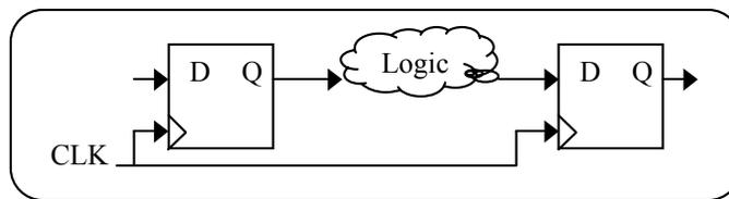
The circuit contains register 1 on the left, some random combinational logic, and register 2 on the right. There are two inequalities that must hold in order for this circuit to work.
