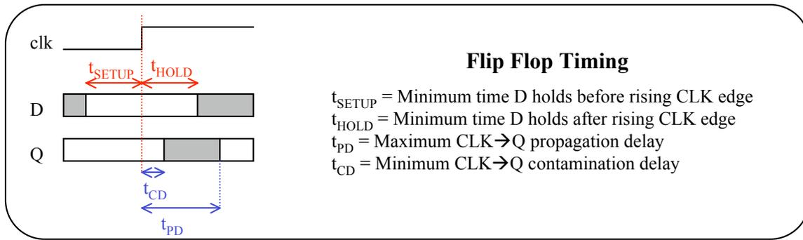
$t_{\text{CD,MASTER}} > t_{\text{HOLD,SLAVE}}$  to ensure that data will not pass through both the master and the slave while both are transitioning. If this inequality does not hold, then you can ensure that the flip flop works by inserting a buffer between the master and slave such that
