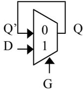
One way to implement the latch is to use a two-input mux. This introduces some timing constraints on the inputs of the latch. The data input D must be valid  $T_{SETUP}$  before G falls and D must stay valid for  $T_{HOLD}$  after G falls.
