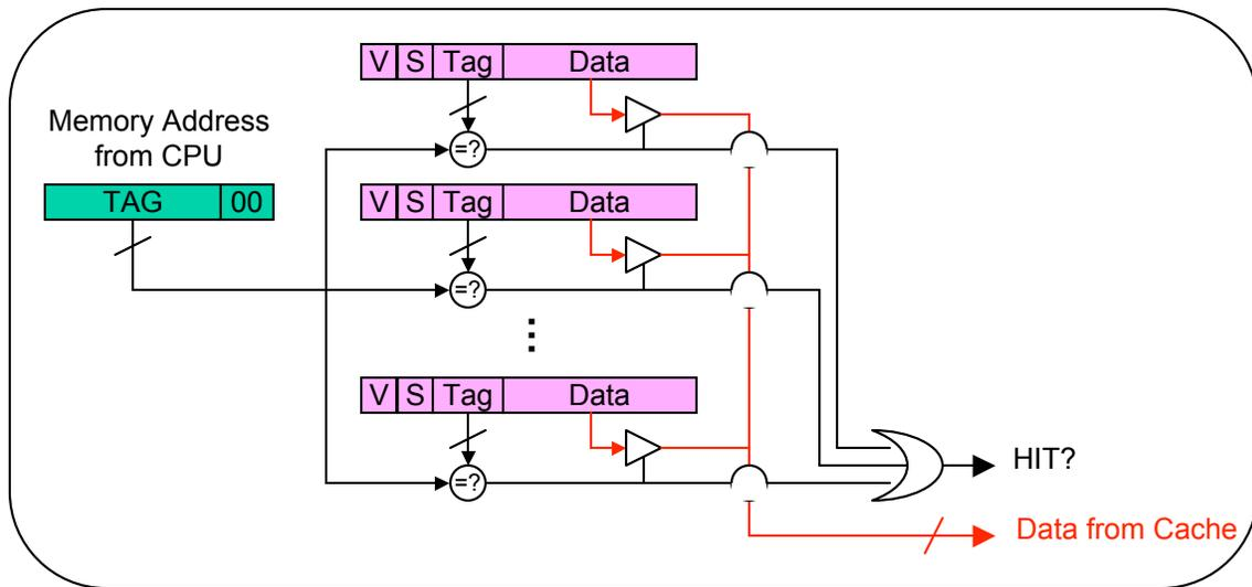
A cache contains many cache lines. A cache line contains (1) a valid bit indicating if the data in that line is valid, (2) optional status bits that indicate if the data is dirty, read-only, etc., (3) a tag formed from the memory address, and (4) the data corresponding to that address.
