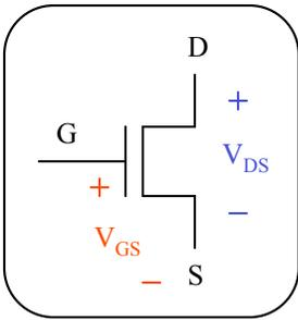
A NFET can be categorized into three “analog” regions – cutoff, linear, and saturation - and two “digital” regions – on and off.
