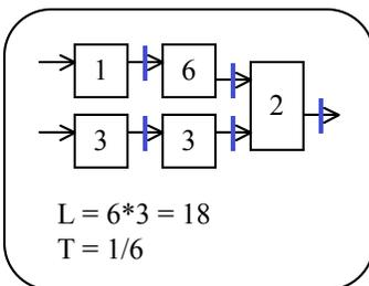
Pipelined circuits contain **registers** in-between the logic blocks. For simplicity, we assume that these are ideal registers with zero contamination and propagation delay, and zero setup and hold time. The register's clock cycle  $t_{CLK}$  is equal to the propagation delay of the slowest block.
