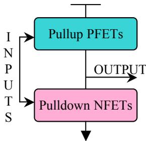
A CMOS Logic gate consists of a bunch of PFETs in the pullup (between power and the output), and a bunch of NFETs in the pulldown (between the output and ground).
