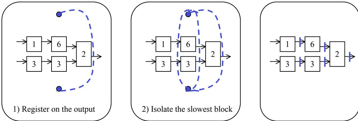
The example above is one of many ways to pipeline this circuit. Any configuration is valid as long as there are an equal number of registers on each path from input to output.
