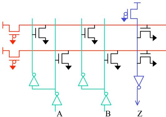
A Read-Only Memory and a Programmable Logic Array consist of **address input lines**, **word lines**, and **bit lines**. You can add NFETs to configure the ROM or PLA to perform many functions. Each word line and bit line is driven by a weak PFET whose input is tied to ground. The weak PFET serves to drive the wire high when there is no path to ground, but is easily overpowered by a NFET.
