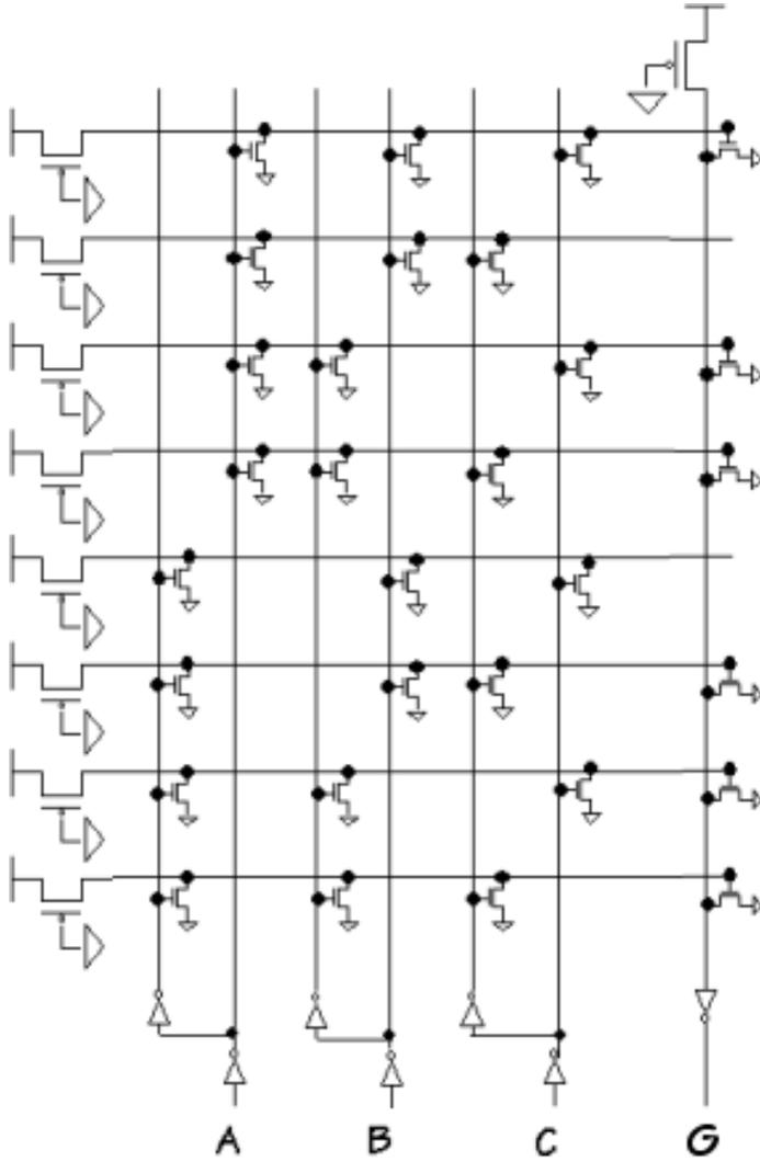
**Problem 9.** Digital Widgets Co. has introduced a new logic IC consisting of two comparator cells in a 14-pin package. A comparator cell, as drawn below, has four inputs and two outputs.
