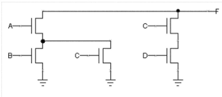
A. Draw a circuit diagram for the pullup circuitry that would complete the static CMOS implementation of  $F(A,B,C,D)$ .
