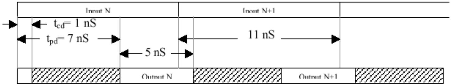
Thus if the inputs transition no faster than every 11 ns ( $\sim 90 \text{ MHz}$ ), the outputs will be stable for at least 5 ns.
