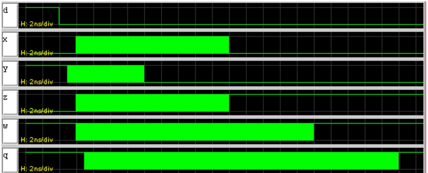
Waveforms with lenient gates:
