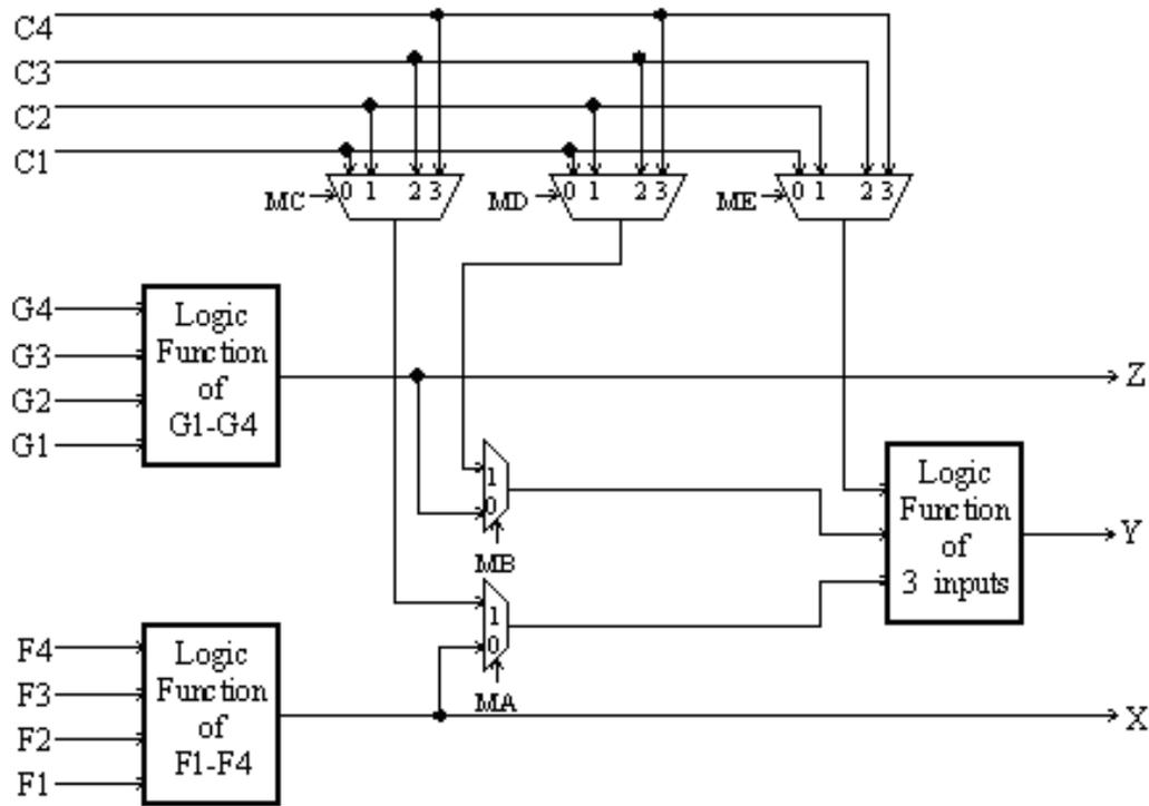
There are two 4-input function generators and one 3-input function generator, each capable of implementing an arbitrary Boolean function of its inputs.
