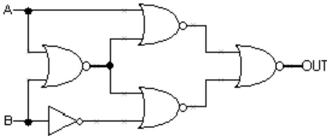
A. ★ What is  $t_{pD}$  for this circuit?
