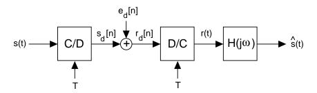
Figure 4-1: Model for A/D-D/A cascade with input s(t) and output r(t). The post-cascade filter  $H(j\omega)$  is used to reduce the effect of quantization noise.
