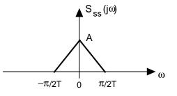
Figure 4-2: Power spectral density of s(t).
