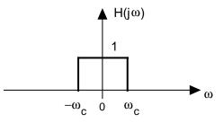
Figure 4-3: Frequency response of the ideal low-pass filter.
