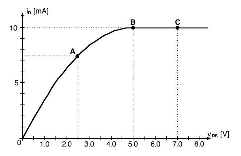
(a) [4 pts] Given that  $V_T = 1$  V, what is the gate voltage  $V_{GS}$  that must be applied to obtain the characteristic shown above?
