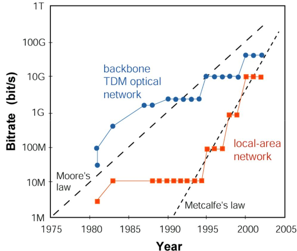
In last 20 years, communication bandwidth through a single optical fiber has increased by ten-thousand fold.
