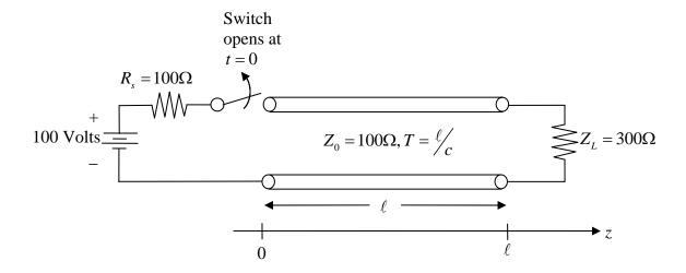
A transmission line of length  $\ell$ , characteristic impedance  $Z_0=100\Omega$ , and one-way time of flight  $T=\frac{\ell}{c}$  is connected at z=0 to a 100 volt DC battery through a series source resistance  $R_s=100\Omega$  and a switch . The  $z=\ell$  end is loaded by a  $300\Omega$  resistor.
