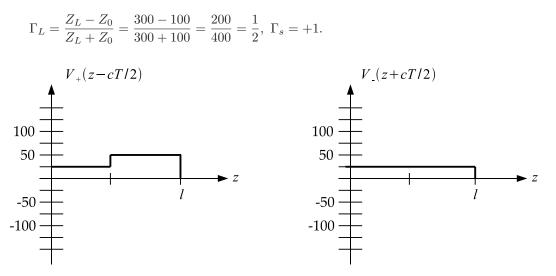
II. Plot the transmission line voltage v(z,t) as a function of z at time t = T/2. Solution:
