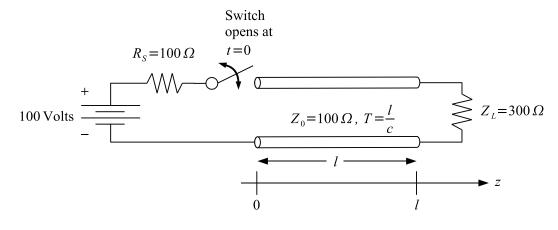
A transmission line of length l, characteristic impedance  $Z_0 = 100 \ \Omega$ , and one-way time of flight T = l/c is connected at z = 0 to a 100 volt DC battery through a series source resistance  $R_s = 100 \ \Omega$  and a switch. The z = l end is loaded by a 300  $\Omega$  resistor.
