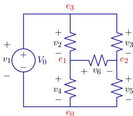
Answers:  $v_1 = e_3 - e_0$ ;  $v_2 = e_3 - e_1$ ;  $v_3 = e_3 - e_2$ ;  $v_4 = e_1 - e_0$ ;  $v_5 = e_2 - e_0$ ;  $v_6 = e_1 - e_2$ ;
