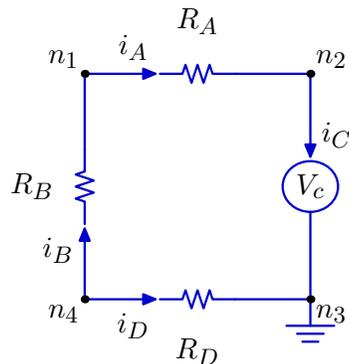
Ultimately, we can find that  $i_A = i_B = i_C = -0.025\text{A}$ ,  $i_D = 0.025\text{A}$ ,  $v_1 = 7.5\text{V}$ ,  $v_2 = 10\text{V}$ , and  $v_4 = 2.5\text{V}$ . Verify this solution by writing out the equations and solving them using a process similar to the one outlined above.
