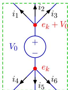
A consistent set of equations can be derived by treating the entire voltage source as a single node, represented by the dashed green box above. The KCL equation for that node,
