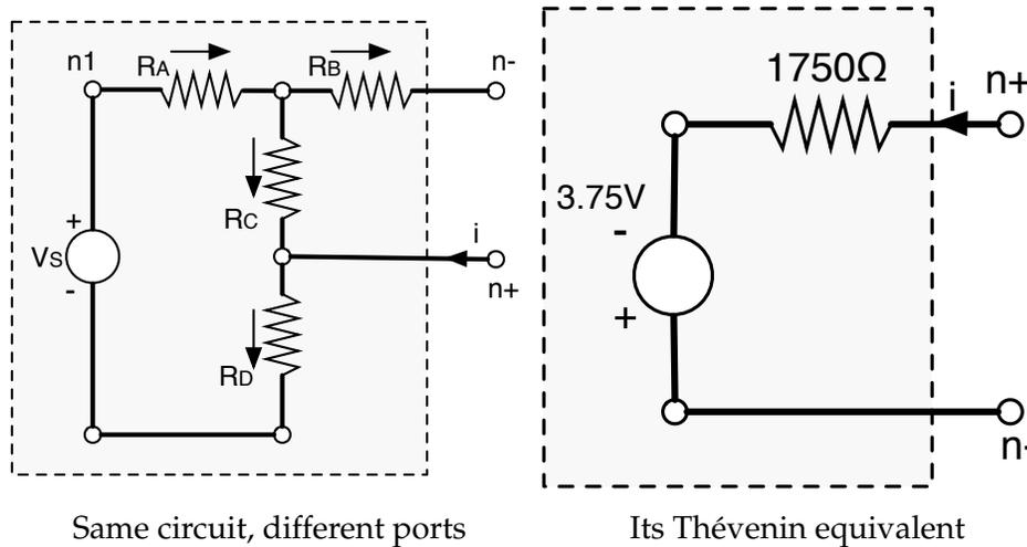
Note also that the top lead is marked  $n_-$  and the bottom one  $n_+$ . If we solve, using the same values for the resistors and voltage source as before, we find that  $V_{th} = -3.75V$  and  $R_{th} = 1750\Omega$ . We show the Thévenin equivalent circuit next to the original. We've changed the polarity of the voltage source and made it 3.75V (instead of having the + terminal at the top and a voltage of -3.75), but that's just a matter of drawing.
