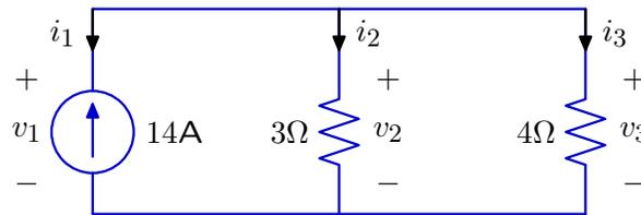
There is a single independent KCL equation:  $i_1 + i_2 + i_3 = 0$ . There are two independent KVL equations that together yield  $v_1 = v_2 = v_3$ . Thus, KCL and KVL together yield three equations in six unknowns. We need three more equations — one from each element. From the current source constitutive relation we have  $i_1 = -14\text{A}$ . From the resistor constitutive relations we have  $v_2 = 3\Omega \times i_2$  and  $v_3 = 4\Omega \times i_3$ . Solving
