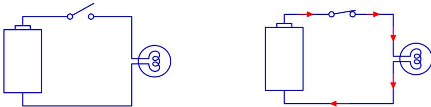
Three parts of the flashlight comprise the circuit: the battery, which supplies power, a bulb, which produces light when connected to the battery, and a switch, which can either be on (connected) or off (disconnected). The important feature of this circuit is that electrical currents flow through it in a loop, as illustrated in the right part of the figure above.
