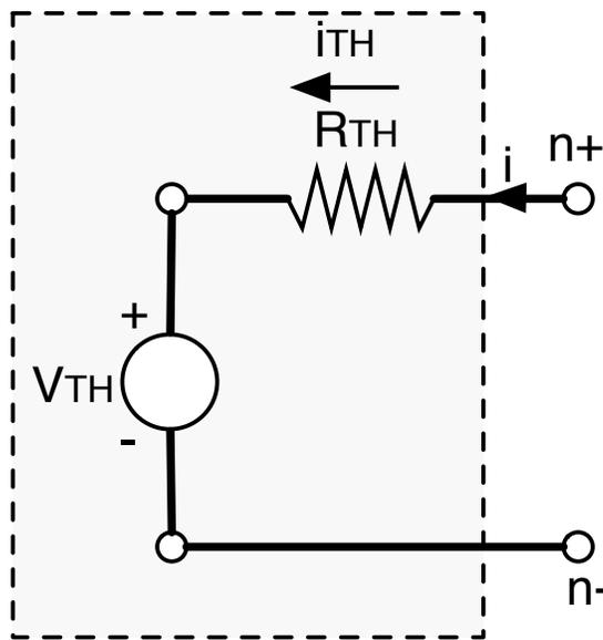
Here, we show a picture of a black (well, gray) box, abstracted as being made up of a circuit with a single voltage source  $V_{th}$  and a single resistor  $R_{th}$  in series. The open-circuit voltage from  $n_+$  to  $n_-$  is clearly  $V_{th}$ . The short-circuit current  $i_{sc}$  (in the direction of the arrow) is  $-V_{th}/R_{th}$ . So, this circuit would have the desired measured properties.<sup>42</sup>
