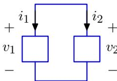
*Example 6.* List all of the KCL and KVL equations for this circuit. There are two nodes in this circuit. As we saw in [Teach Yourself 2](#), this implies that there is a single independent KCL equation, which is  $i_1 + i_2 = 0$ . There is a single loop and therefore a single KVL equation:  $v_1 - v_2 = 0$ . Thus we have four unknowns and just two equations. More information is needed to solve for the currents and voltages.
