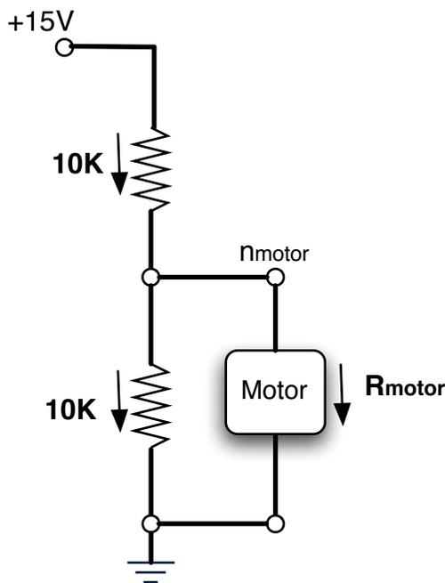
But what will the voltage  $v_{motor}$  end up being? It all depends on the resistance of the motor. If the motor is offering little resistance, say  $100\Omega$ , then the voltage  $v_{motor}$  will be very close to 0.<sup>43</sup> So, this is not an effective solution to the problem of supplying 7.5V to the motor.
