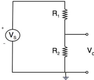
1. For a given set of values for  $R_1$  and  $R_2$ , if  $R_2$  is then increased, will the voltage  $V_o$  increase or decrease? (Enter either *increase* OR *decrease*)
