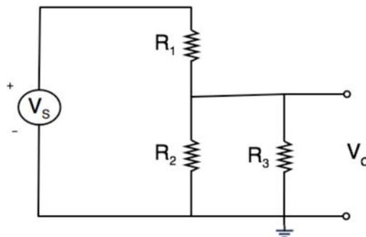
Note that the only difference between this circuit and the one in the previous part is the addition of  $R_3$ . We are interested in the effect on  $V_o$  of adding this resistor. Call the voltage across  $R_2$  when  $R_3$  is not present  $V_d$ . Assume  $R_1$  and  $R_2$  are 1000 Ohm.
