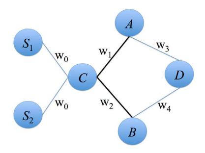
*Goal:* To ensure that the links connecting C to A and C to B, shown as darker lines, carry *equal traffic load.* All the traffic is generated by S1 and S2, in some unknown proportion. The rate (offered load) at which S1 and S2 together generate traffic for destinations A, B and D are R\_A, R\_B, and R\_D, respectively. Each network link has a bandwidth higher than R\_A + R\_B + R\_D. There are no failures.
