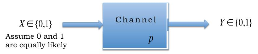
With probability p the input binary digit gets flipped before being presented at the output.
