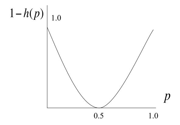
For low-noise channel, significant reduction in uncertainty about the input after observing the output.
