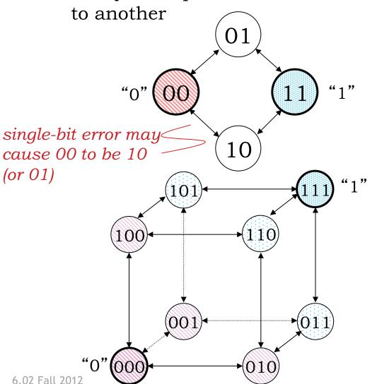
Code: nodes chosen in hypercube + mapping of message bits to nodes
