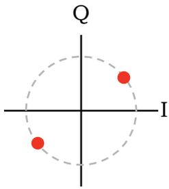
In bipolar modulation ( $x[n]=\pm 1$ ), also called Binary Phase Shift Keying (**BPSK**) since the modulated carrier changes phase by  $\pi / 2$  when  $x[n]$  switches levels, the received constellation will be rotated with respect to the transmitter's constellation. Which phase corresponds to which bit?
