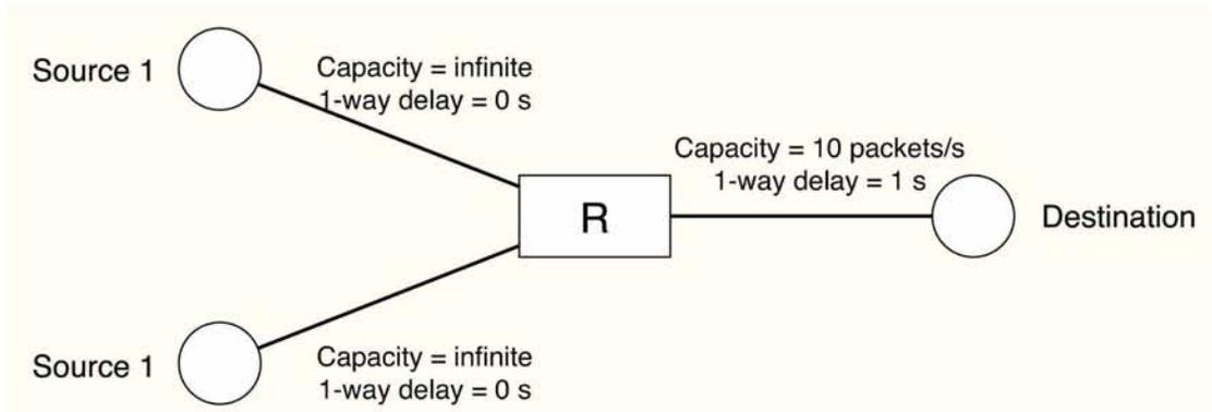
**6. [6 points]:** Assume the window size is fixed and only Source 1 is active, whereas Source 2 does not send any traffic. What is the smallest sliding window that allows Source 1 to achieve the maximum throughput?
