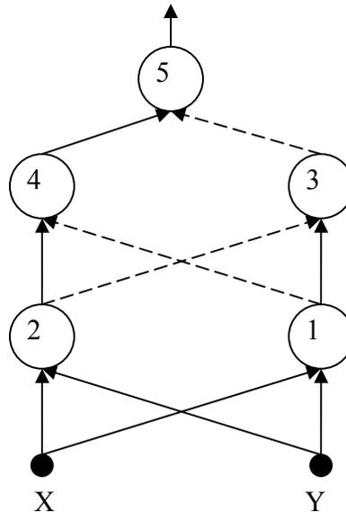
In this network, **all the units are sigmoid except unit 5 which is linear** (its output is simply the weighted sum of its inputs). All the bias weights are zero. The dashed connections have weights of -1, all the other connections (solid lines) have weights of 1.
