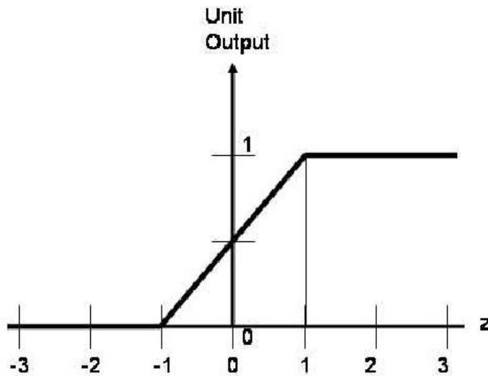
$$\begin{aligned} f(z) &= 0 && \text{if } z < -1 \\ f(z) &= 1 && \text{if } z > 1 \\ f(z) &= 0.5(z + 1) && \text{otherwise} \end{aligned}$$
