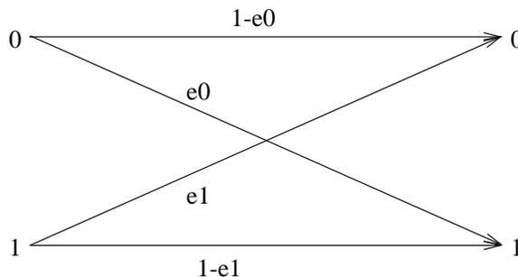
Figure 1: Error probabilities in a binary communication channel.
