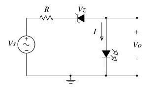
This circuit is constructed with a Zener diode an LED, a resistor and a voltage source.
