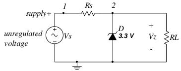
The supply is able to provide a maximum current of 1.5A, and the Zener diode has an effective resistance of  $30\Omega$ .
