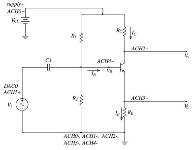
Build the circuit with  $R_1 = 20k\Omega$ ,  $R_2 = 5k\Omega$ ,  $R_C = 5k\Omega$ ,  $R_E = 1k\Omega$ , Vcc = 10V. These values should give a Q-point:  $I_{CQ} = 1.3mA$ ,  $V_{CEQ} = 2.5V$  For  $V_{CC}$  use the variable power supply and set the voltage to 10 Volts. The signal Vi is available at DACO.
