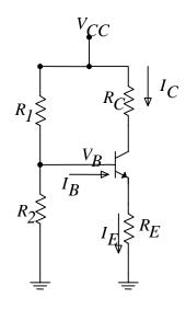
• For  $R_1 = 20k\Omega$ ,  $R_2 = 5k\Omega$ ,  $R_E = 1k\Omega$ , Vcc = 10V, determine resistor  $R_C$  so that the transistor enters saturation.
