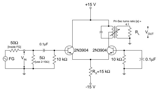
Figure 2: Cascode amplifier circuit driving resonant IF transformer.
