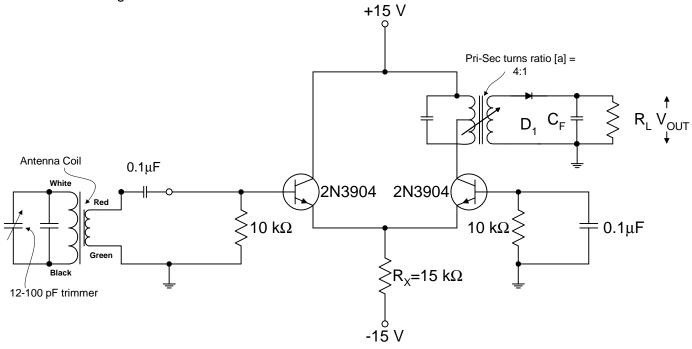
Figure 8: Resonant antenna/antenna coil connected to IF amplifier.
