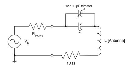
Figure 7: Antenna tuning circuit for transmitting AM carrier from function generator.
