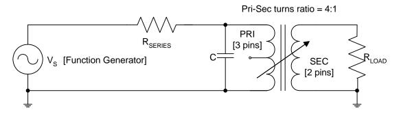
Figure 1: Circuit for parallel resonance, Experiment 1.
