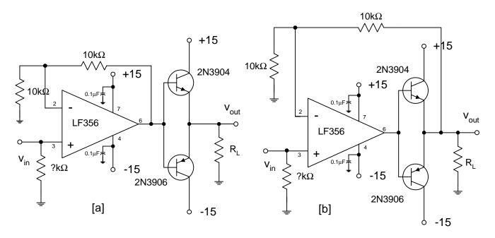
Figure 5: Push-pull output stage circuits.
