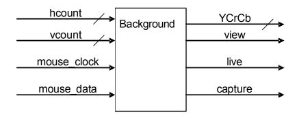
Background takes care of most of the user interface items appearing on the monitor. This includes the white frames surrounding the video display and buttons, and the mouse cursor. To create a border, Background simply instantiates four instances of the module
