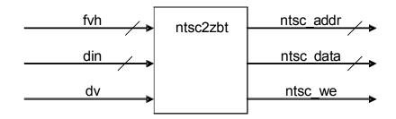
The ntsc2zbt module prepares the NTSC data received from the NTSC decoder and loads into the ZBT SRAM so that it can be displayed. The timing issue in this module are not trivial as video data is coming in from the NTSC at a different rate that the video data is being written to memory, and also at a different rate as the SRAM clock. To remedy this, the ntsc2zbt module uses a series of pipelines to determine when and where data should be written to the zbt SRAM.
