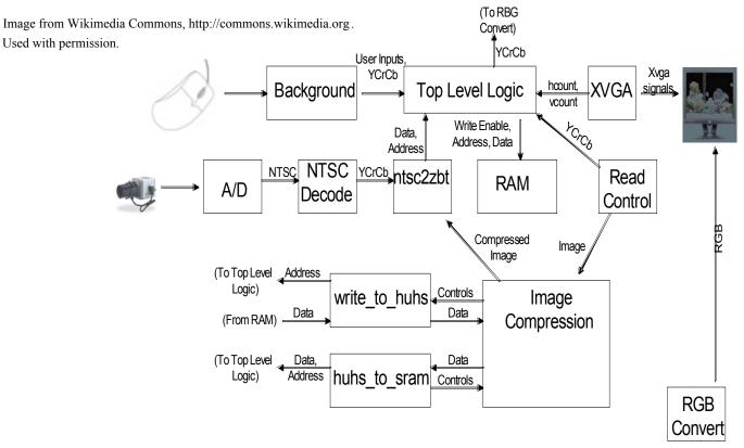
Figure 4: Digital Camera Block Diagram
