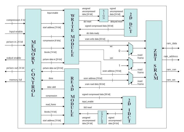
Figure 7: Image Compression & Storage Block Diagram
