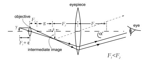
Figure 1: Ray diagram for a microscope
