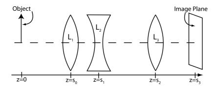
Figure 2: Diagram of a three-lens imaging system, with a biconcave thin lens between two biconvex thin lenses.
