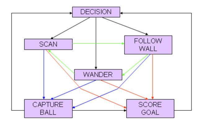
Because the algorithms for finding balls and finding goals are so similar, we also decided to incorporate two modes into our finite state machine. The default mode is Ballmode, while the other is Goalmode. On the model, the green arrows represent changes of state from our timing out mechanisms, the red arrows account for the recognition that the robot has found a ball, and the blue arrows depict changes of state that result from the recognition that the robot has found a goal.
