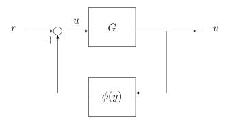
Figure 2.1: Feedback setup for Problem 2.1
