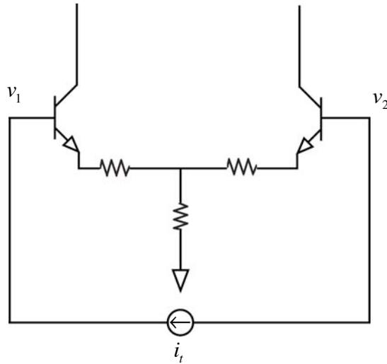
$$v_1 = i_t R_{HALF} \rightarrow v_t = v_1 - v_2 = 2i_t R_{HALF} \rightarrow R_{IN} = 2R_{HALF}$$
