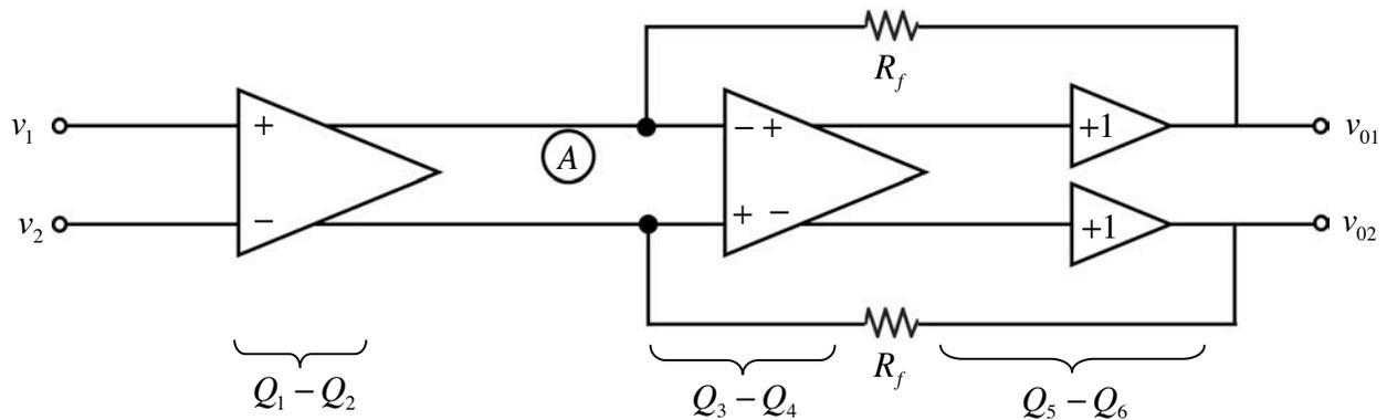
If we look in the course reader, we'll see that the gain of the amplifier formed by  $Q_3 - Q_4$  is on the order of 100. The data sheet specs the output swing at  $V_{p-p}$ . What this means is that the differential voltage swing at point (A) is only  $47mV_{p-p}$  ... it is a low-swing node!
