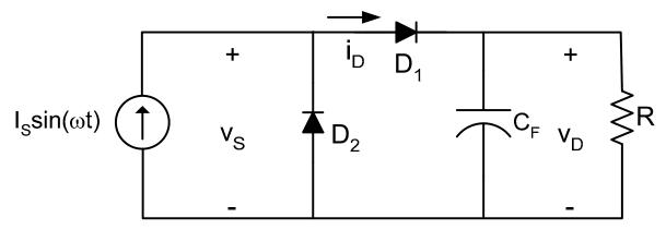
Figure 1.2 A half-wave rectifier driven from a sinusoidal current source.
