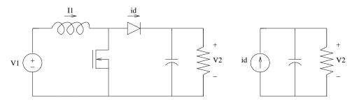
Figure 5.22: Boost Converter Ripple
