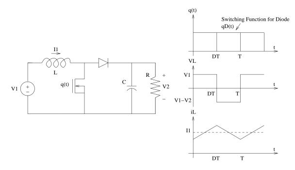
Figure 5.28: Boost Converter Waveforms
