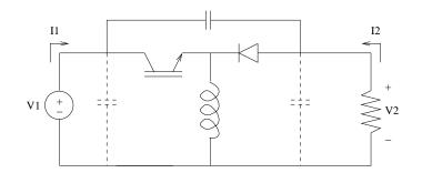
Figure 5.16: "Buck/Boost" or "up/down" converter
