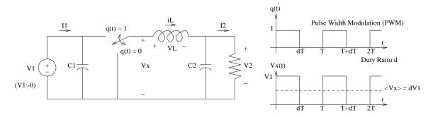
Figure 5.3: DC/DC Converter
