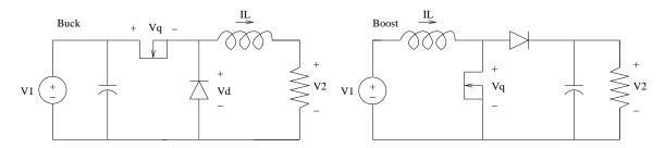
Figure 5.21: Direct Converters (neglecting ripple)
