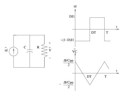
Figure 5.24: Ripple Model with Capacitor
