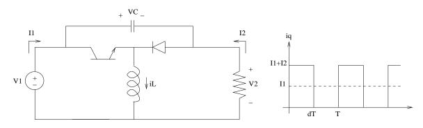
Figure 5.20: Indirect Converters (neglecting ripple)
