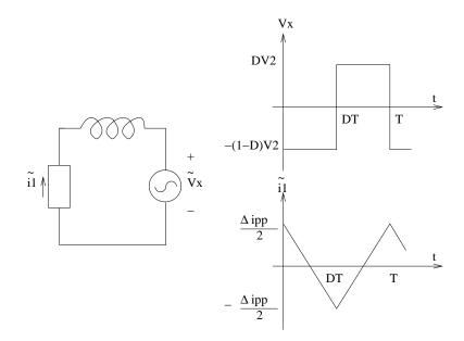
Figure 5.26: Ripple Model with Inductor
