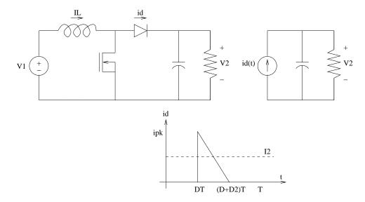
Figure 5.31: DCM Operation Model
