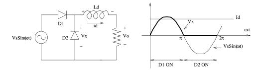
Figure 2.1: Simple Half-wave Rectifier
