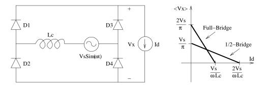
Figure 2.8: Full-Bridge Rectifier
