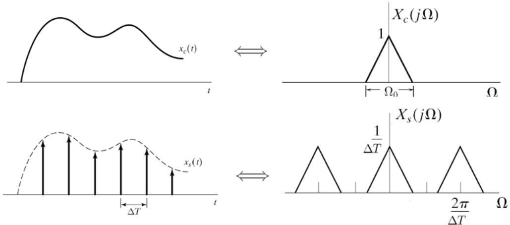
Sampling in time corresponds to replication in the frequency domain. In order to recover  $X_c(j\Omega)$  perfectly by low-pass filtering  $X_s(j\Omega)$ , frequency aliasing should be avoided. Therefore,  $x(t)$  should be bandlimited to  $\Omega_0$ , and sampling interval should be short enough so that
