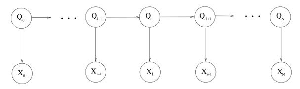
Assume that, in each frame,  $Q_i$  is discrete with cardinality 4,  $X_i$  is continuous and one-dimensional, and  $p(x_i|q_i)$  is a mixture of up to  $M_{q_i}$  Gaussians, i.e.
