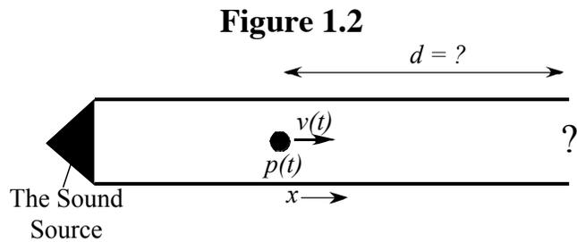
while to the right:  $d$ , the distance between the measurement point and the termination, and the status of the termination of the tube varies. The system is in the steady state.
