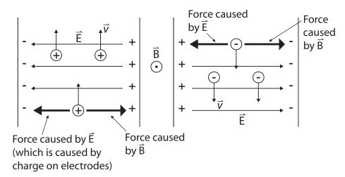
Figure 1: Figure for 1C. Opposite polarity voltages between holes and electrons (Image by MIT OpenCourse-Ware.)
