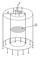
Figure 2: Figure for Problem 1.3 Part A. A cylinder with volume current going in the +z direction for r < b. (Image by MIT OpenCourseWare)
