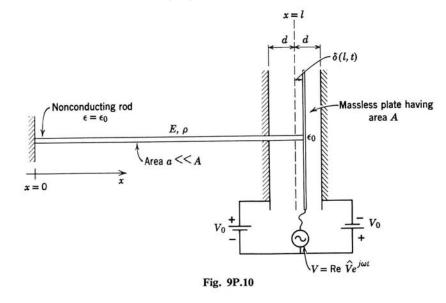
Figure 4: A long thin rod fixed at x = 0 and driven by imposed voltages at  $x = l + \delta(l, t)$ Courtesy of Herbert Woodson and James Melcher. Used with permission. Woodson, Herbert H., and James R. Melcher. *Electromechanical Dynamics, Part 2: Fields, Forces, and Motion.* Malabar, FL: Kreiger Publishing Company, 1968. ISBN: 9780894644597.
