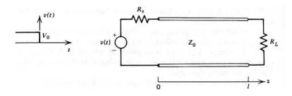
Figure 6: Transmission line system.
