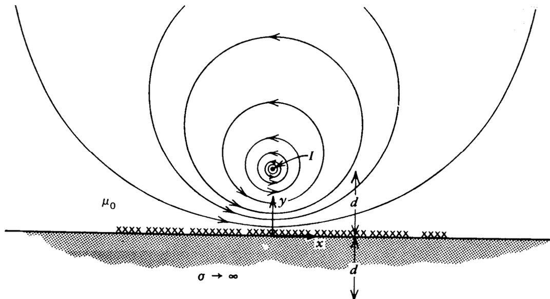
A line current  $I$  of infinite extent in the  $z$ -direction is at a distance  $d$  above a perfectly conducting plane.
