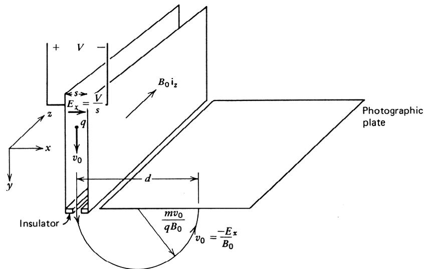
The mass spectrograph uses the circular motion to determine the masses of ions and to measure the relative proportions of isotopes. Charges enter between parallel plate electrodes with a  $y$  directed velocity distribution. Gravitational effects are negligible compared to the electric/magnetic forces since the ions have so little mass.
