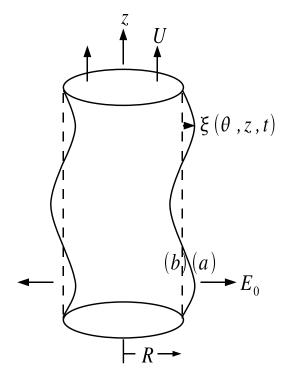
Figure 1: A cylindrical liquid column of equilibrium radius R moves with velocity U in the z direction and has a radial electric field for  $r > R + \xi(\theta, z, t)$  (Image by MIT OpenCourseWare.)
