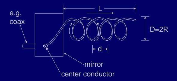
Waves add in phase in the forward direction if If L >> D, standing wave at end is small because of radiation losses. Assume ~ TEM propagation
