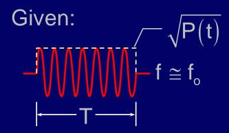
CW transmitted pulse at  $f_o$ , power = P(t)
