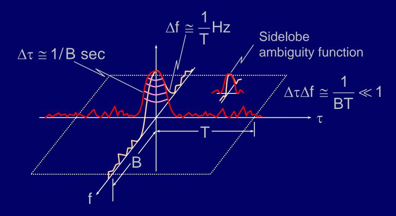
Design of  $s(t) \cos \omega t$  to yield minimum ambiguity sidelobes is difficult; trial and error is common design technique.
