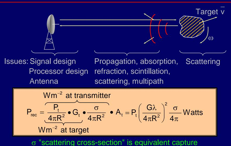
cross-section for a target scattering isotropically
