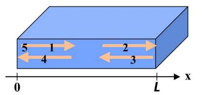
For sustained lasing we must have the intensity after a full circuit (5) be equal to, or greater than, the initial intensity (1):  $R_1 R_2 I_o e^{(g-\alpha_l)2L} \ge I_o$
